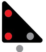
Structure in night-time operation or network malfunction
