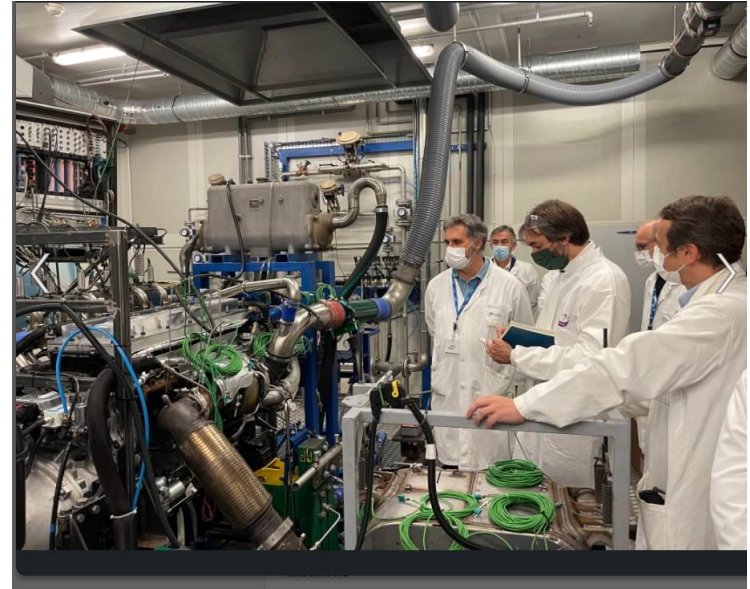
MH8 Engine being tested on test bench
