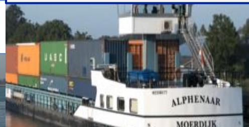
First vessel with exchangeable ZES battery containers for propulsion (NL)
